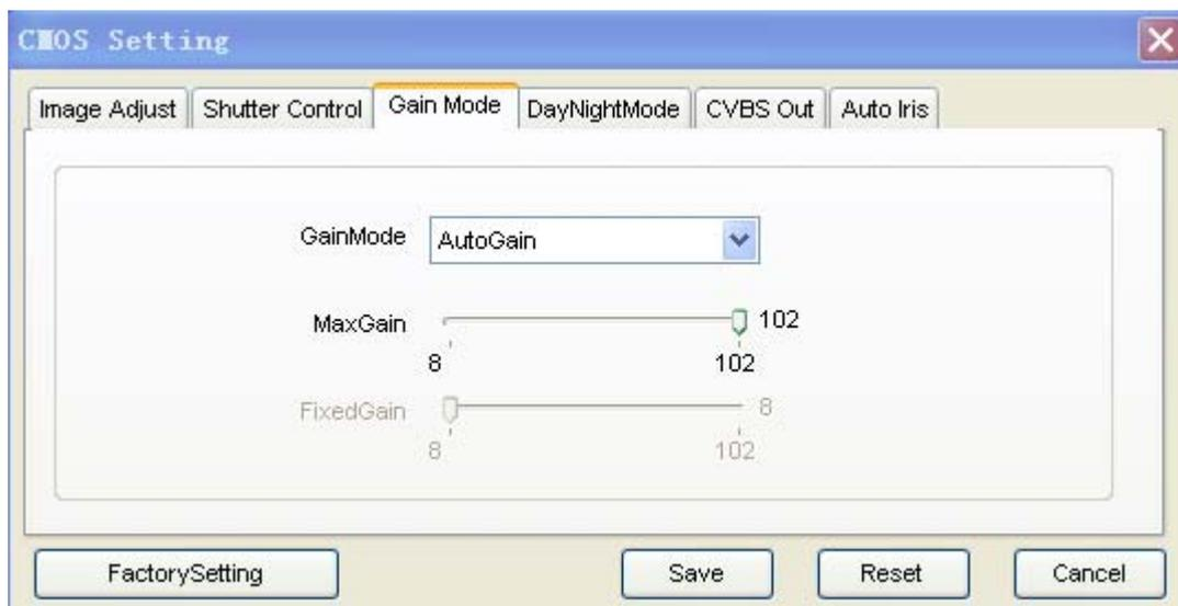
Gain mode includes AutoGain and fixedGain, MaxGain is adjustable to meet different conditions.
