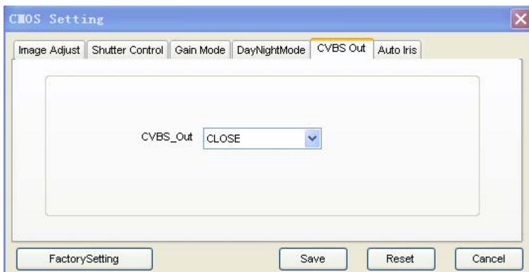
When CVBS\_Out open, cameras support analogue BNC output, the default is CLOSED.
