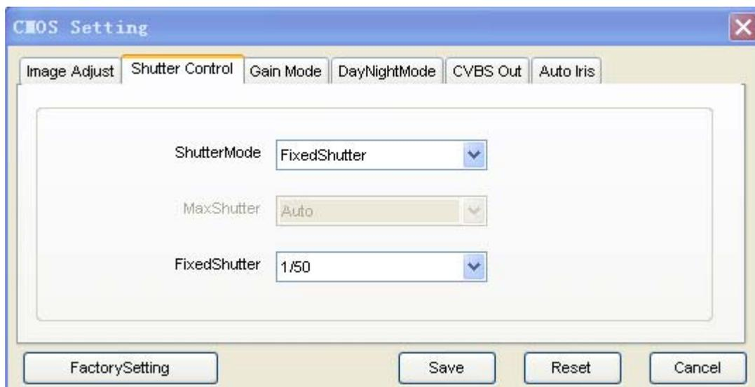
Shutter mode includes 2 modes: fixed and auto shutter. choose "on", shutter adjusts automatically during the max and min; choose "off", fixed shutter is available to be adjusted.
